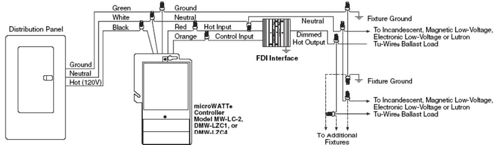
Figure 3 – Wiring the FDI Interface with PerSONNA® Controller models PN-IR or PN-IR-LP
